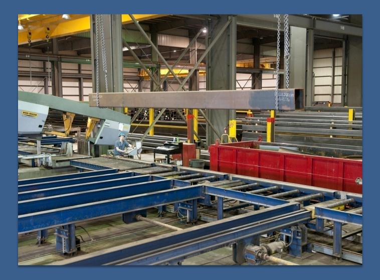
One 18" Vertical Saw, miter cut up to 45 degrees Two 25" Horizontal Saws, miter cut up to 45 degrees Two 42" Horizontal Saws
