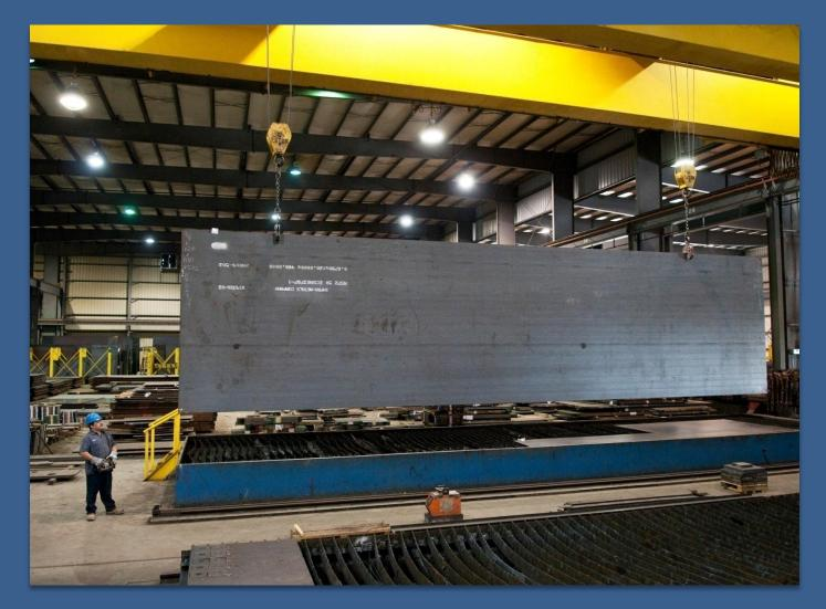
•Burns .050" through 1" thick plate Capable of holding two 120"x240" plates at one time
